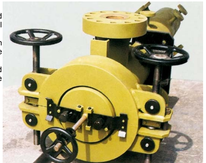
Fig. 7: High pressure opening closure for FLO-GAS filter.
